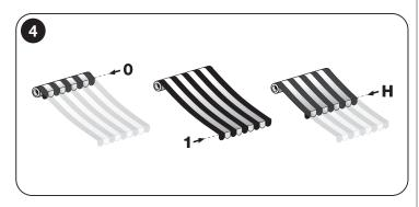
When the limit switches are not programmed yet, the awning can be moved only in the "hold-to-run" mode, i.e. keeping the control key pressed for the desired duration of the manoeuvre; the movement stops as soon as the user releases the key. However, after programming the limit switches, <u>briefly pressing the appropriate key</u> will start the awning and it will stop moving automatically as soon as the awning reaches the required position.
